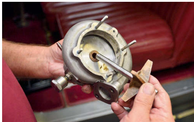
...to reveal a broken impellor shaft. A new one is on order and will be fitted, with the vehicle tested, before it is offered for sale.
