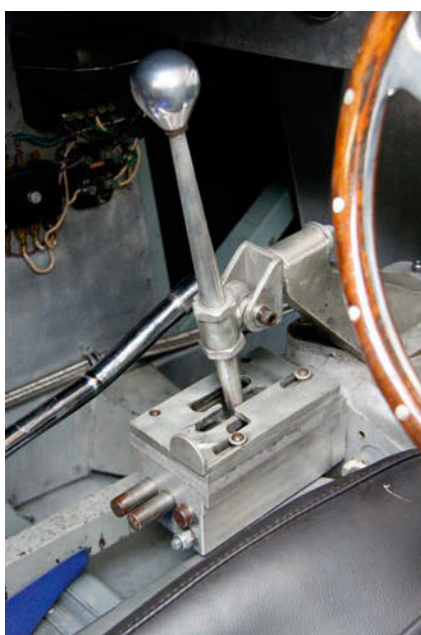
Beautifully machined gear selection, linking to R Type transmission.
