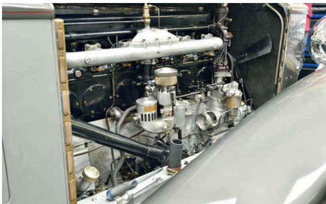
All vehicles get a full PDI: this model suffering from overheating and so the water pump was removed...
