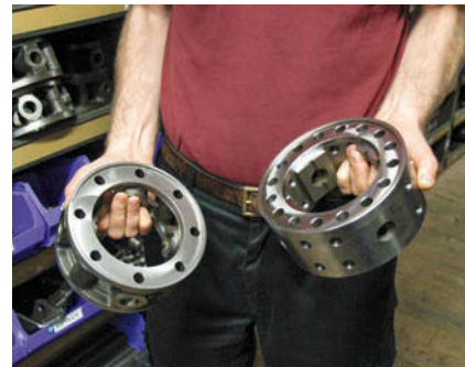
William Medcalf builds modern day parts for its historic racers. Benchmark competition diff (right) alongside standard version.
