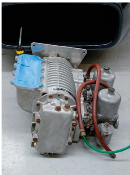
The original Rootes type Allard supercharger has been kept with the vehicle all its life and will be reunited at a later date.
